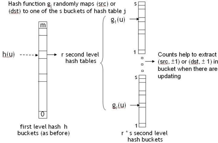
Fig. 3. CBF to count network packet.
