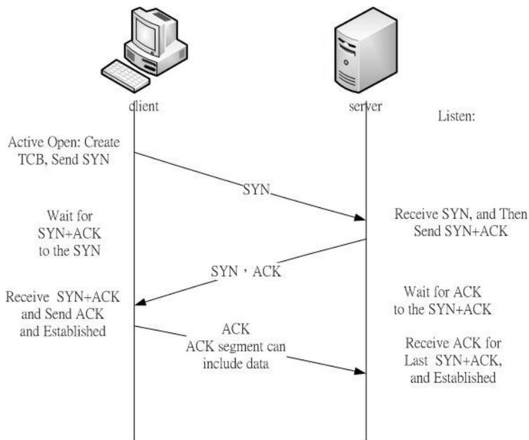
Fig. 1. Three-way handshake.
